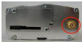
For Simplekey units supplied within a KMS metal cabinet or mounted upon a KMS chassis and/or within an OEM cabinet, the power lead and serial lead will already be connected to the Simplekey door controller and only the antenna connection will need to be made.
