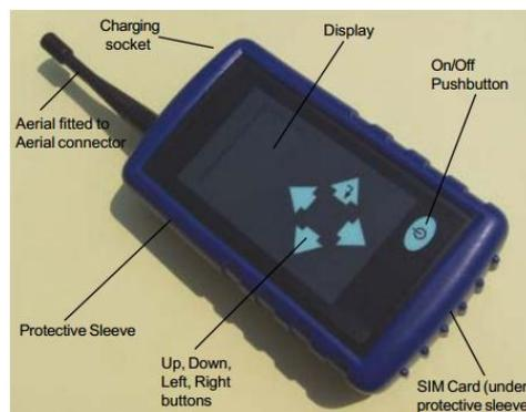
The external aerial can be connected via the aerial connector and positioned in various locations in order to select the most suitable. If no SIM card is fitted the unit will search for all network providers. You may well find that one a particular network provider has a strong signal in one location but a poor signal in another and if a suitable aerial location can't be found for your preferred provider, then an alternative may need to be used.
